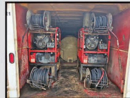
(4) Enclosed Steamers Trailer with 2 Hotsy 3000 PSI Units
